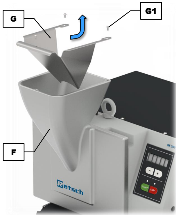
Fig. 25: Cleaning the feed hopper
