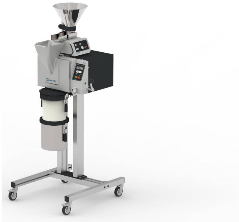
Fig. 30: SK 300 with vibratory feeder DR 100
