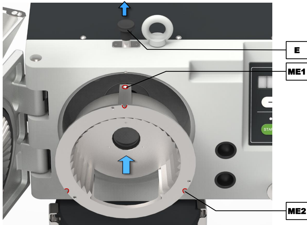
Fig. 17: Inserting the grinding insert
