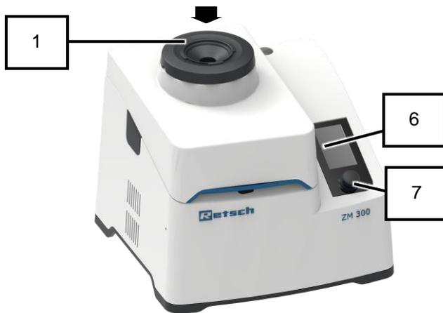
1. Set the parameters for grinding on the touch display (6) and with the control dial (7).
