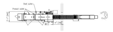
OptiBreaker Basic 5/6 - Inclined Roller Table - FlexLoader 5/6 with Destacker
