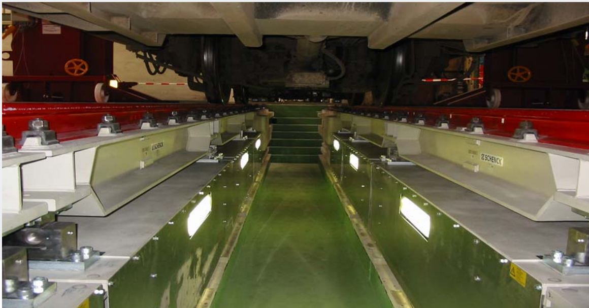
Picture showing a system for an entire vehicle, where each measuring rail can be adjusted along the z-axis to simulate a correction of wheel load distribution
