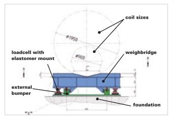
Fig. 14: Basic structure of a legal-for-trade coil scale 35t
