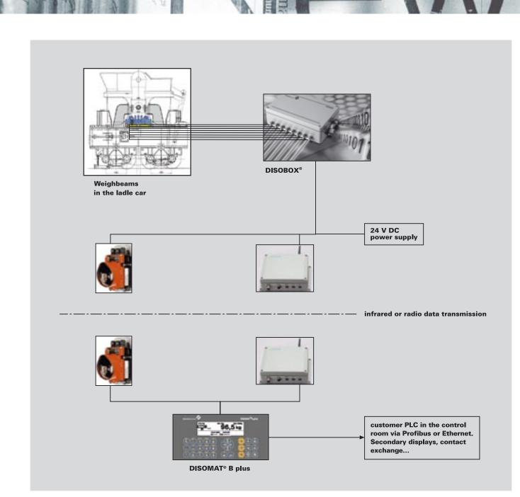
Figure 19. Application example for a ladle transfer car weighing electronics
