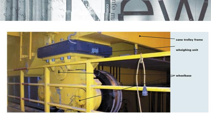
Fig. 6: Weighing unit of a 400t ladle transport crane (Courtesy: Siemens VAI)
