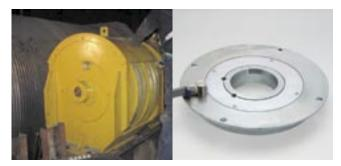
Fig. 8: New upper sheave block 350t with pre-assembled DRAsensors (Courtesy: Ternium Sidor), Fig. 9: Schenck Process Radial Force Sensor DRA
