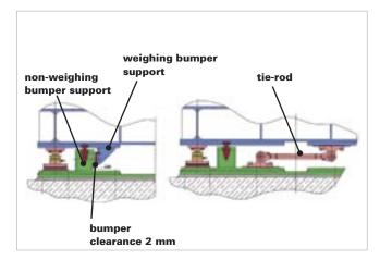
Fig. 15: Bumpers for horizontal load transmission, Fig. 16: Tie-rods for horizontal load transmission
