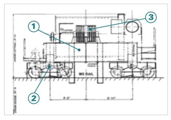
Fig. 4: Installation places for a weighing system inside the trolley of a ladle transport crane
