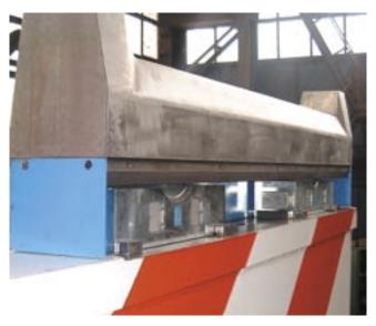
Fig. 2: Weighing unit of a 350t ladle turret (Courtesy: Siemens VAI)
