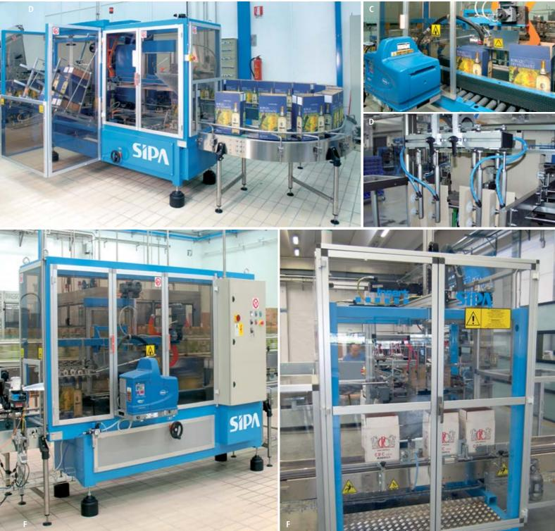
A) Formex carton magazine B) Formex: overall view C) Stick: sealer and carton sealing detail D) Insert: detail of the partition inserting portal with double head E) Stick: overall view F) Insert: overall view
