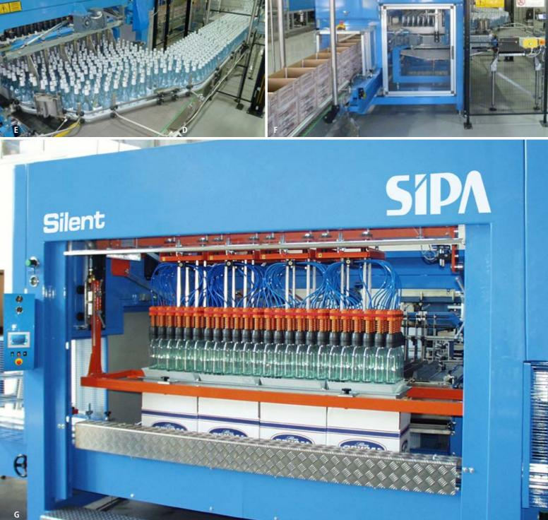
A) Silent: pneumatic membrane gripping heads B) Jolly: overall view C) Jolly: double vacuum head for small size bottles D) Jolly: adjustable pneumatic membrane gripping heads E) Silent: orthogonal bottle feeding F) Silent: carton feeding G) Silent: overall view
