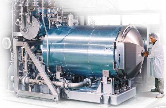
A revolution in the industry, the Steriflow® Shaka®\* represents a new generation of autoclaves. With its patented high-frequency shaker system, the sterilization cycle is 3 to 5 times shorter than any other type of machine. You can access much higher temperature levels with an exceptionally fast heating and cooling period. The result: an enhanced product with better preserved taste and nutritional qualities.
