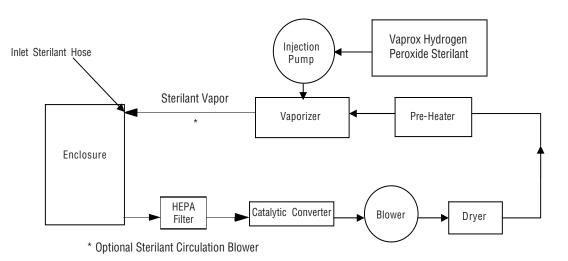
Figure 1 - Typical Closed-Loop Process Diagram
