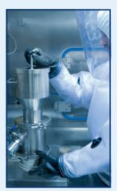
Half suits are available in a range of different materials and are manufactured to high standards providing maximum protection to the operator. In addition fresh air supply to the internal cavity ensures operator comfort at all times.
