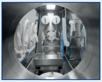
Our sampling and dispensing Isolators guarantee OEL levels for active pharmaceutical ingredients and potent compounds to  $<1\mu g/m^3$  over a task duration or TWA.
