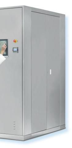
The chamber internal surfaces are insulated and heated by means of separated black steam flowing through a full dimple jacket. Pure steam inlet is controlled with a PID valve and condensates are continuously evacuated of through the drainage offering you **excellent uniformity of temperatures**; better than  $\pm$  0.5°C during all the sterilisation phase. Fulfilling the requirement of EN-285.
