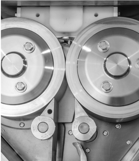
Counter-Rotating Rolls For Precise Controllable Compaction
