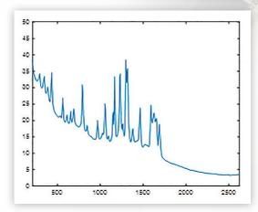
Above, results from the Defender Omega analyzer's analysis of a controlled drug precursor. By subduing fluorescence, spectral peaks become visible, leading to the chemical's identification.
