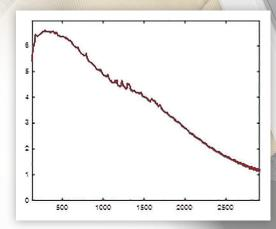
Above, an alternative product's results. Obscured by overwhelming fluorescence, the precursor's spectral peaks are not available for analysis — results are inconclusive.
