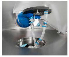
Figure 6. Sparge line support.
