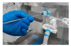
Figure 9. S.U.B. temperature sample port.
