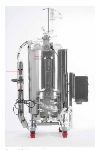
Figure 11. Tubing and cable management tree.
