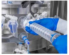
Figure 5. Bioreactor probe assembly.
