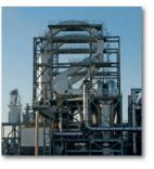
The dryer design is so called a full ring dryer; its working principle is pure convection with short and 'extended short' retention time. The dryer mainly consists of a disintegrator, the drying duct and bend, the manifold, adjustable blades, an external recycling system a filter and fan.
