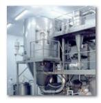
If the starches are further processed and liquid streams as maltodextrin. ysine, etc. are to be dried, VetterTec offers a spray dryer. Spray dryers are pure convection dryers and atomize the
