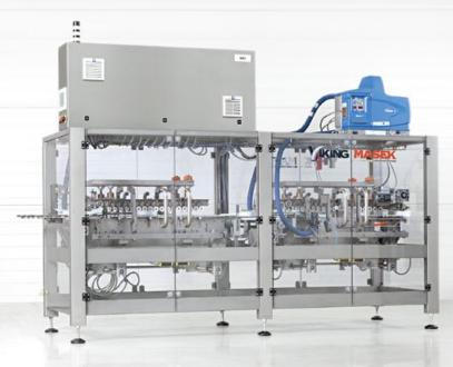
Viking Masek's CLM machines are a family of carton closing machines. We offer straight-line or right-angle units to close one, two or three flaps of the cartons. The unique turning mechanism provides gentle handling of the cartons and of the products inside.
