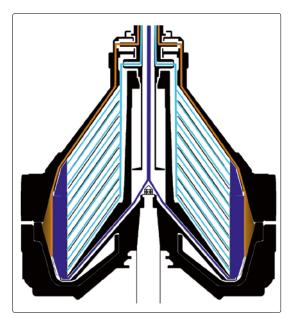
**Fig. 3** The disk stacks in the clarification separator ensure safe bacteria removal from the milk
