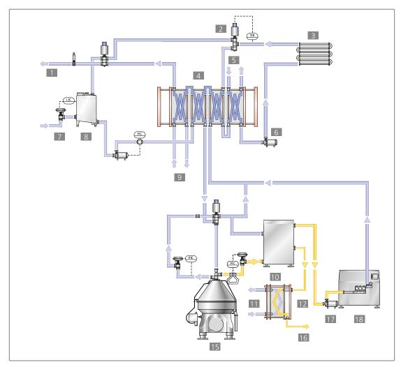
Fig. 1 Conventional process of the milk pasteurization
