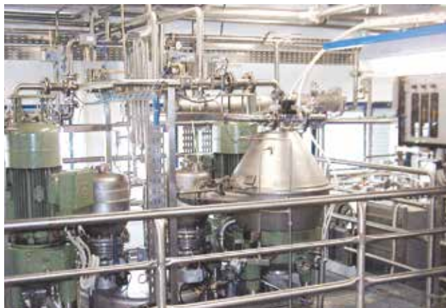
Fig. 14 Installation with type XSC 35 separators
